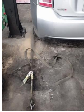
Fig. 7. Security straps and anchoring of the vehicle.
