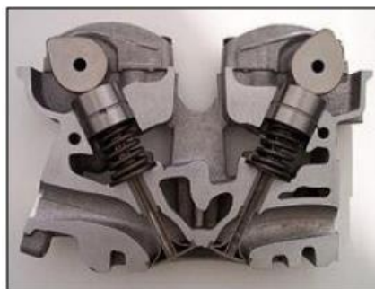
Fig. 2. Camshaft and valve configuration
