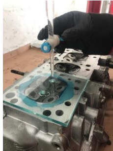
Fig. 1. Measurement of the combustion chamber volume
