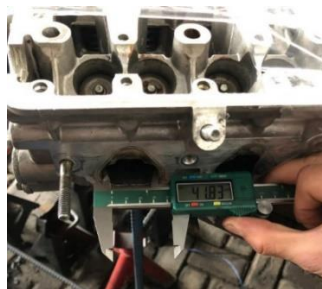
Fig. 3. Measurement of the intake manifold nozzle diameter
